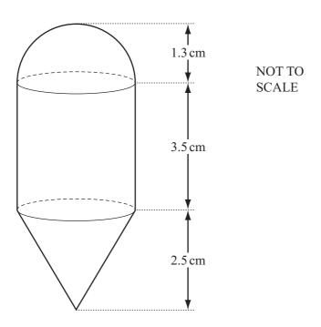
The diagram shows a brass object, used by builders, known as a plumb bob. The plumb bob is made up of a hemisphere, a cylinder and a cone, each of radius 1.3 cm. The height of the cylinder is 3.5 cm and the height of the cone is 2.5 cm.
