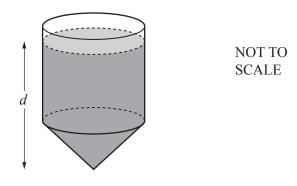
Calculate the depth, *d*, of the water. [The volume, *V*, of a cone with radius *r* and height *h* is  $V = \frac{1}{3}\pi r^2 h$ .]
