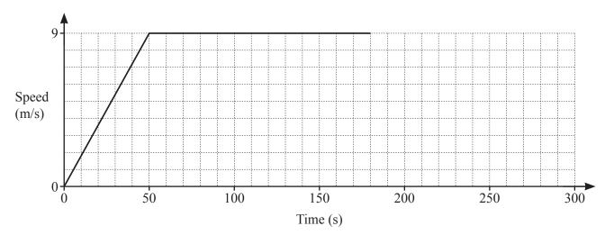
(a) Find the acceleration, in m/s<sup>2</sup>, of the train during the first 50 seconds.
