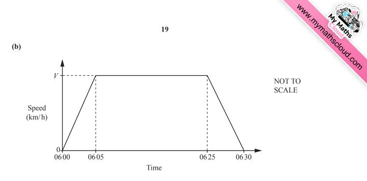
The speed-time graph shows the first 30 minutes of another train journey. The distance travelled is 100 km. The maximum speed of the train is V km/h.
