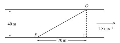
The diagram shows a river with parallel banks. The river is  $40 \,\mathrm{m}$  wide and is flowing with a speed of  $1.8 \,\mathrm{ms^{-1}}$ . A canoe travels in a straight line from a point P on one bank to a point Q on the opposite bank  $70 \,\mathrm{m}$  downstream from P. Given that the canoe takes  $12 \,\mathrm{s}$  to travel from P to Q, calculate the speed of the canoe in still water and the angle to the bank that the canoe was steered.
