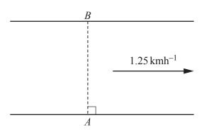
A river flows between parallel banks at a speed of  $1.25 \,\mathrm{kmh^{-1}}$ . A boy standing at point A on one bank sends a toy boat across the river to his father standing directly opposite at point B. The toy boat, which can travel at  $v \, \text{kmh}^{-1}$  in still water, crosses the river with resultant speed 2.73 kmh<sup>-1</sup> along the line AB.
