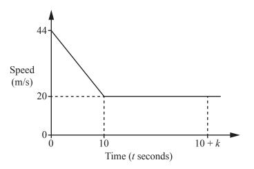
The train slows down uniformly from a speed of 44 m/s to a speed of 20 m/s in a time of 10 seconds. It then continues at a constant speed of 20 m/s.
