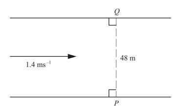
The diagram shows a river with parallel banks. The river is 48 m wide and is flowing with a speed of  $1.4 \text{ ms}^{-1}$ . A boat travels in a straight line from a point P on one bank to a point Q which is on the other bank directly opposite P. It is given that the boat takes 10 seconds to cross the river.
