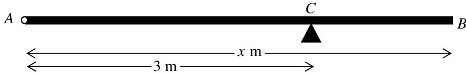
The figure above shows a uniform wooden beam  $AB$ , of length  $x$  m and weight 80 N. The beam is smoothly hinged at  $A$  and rests in a horizontal position on a smooth support at  $C$ , where  $AC = 3$  m.
