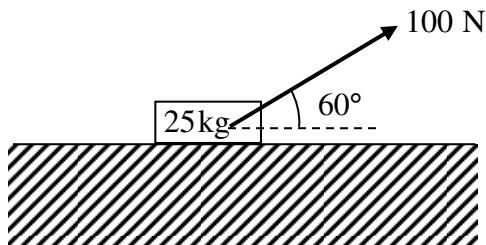
The figure above shows a small box of mass  $25\text{ kg}$ , pulled along rough horizontal ground by a light inextensible rope, which is inclined at  $60^\circ$  to the horizontal.
