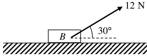
A box  $B$  of mass 1.25 kg is pulled along rough horizontal ground by a force of magnitude 12 N inclined at  $30^\circ$  to the horizontal, as shown in the figure above. The box is modelled as a particle moving on a rough horizontal plane where coefficient of friction between the particle and the plane is 0.25.
