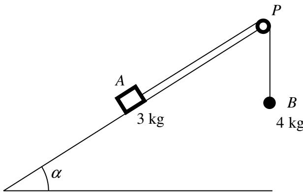
Two particles  $A$  and  $B$ , of mass 3 kg and 4 kg respectively, are attached to each of the ends of a light inextensible string. The string passes over a smooth pulley  $P$ , at the top of a fixed rough plane, inclined at  $\alpha$  to the horizontal, where  $\tan \alpha = 0.75$ .
