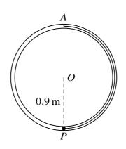
The diagram shows a smooth narrow tube formed into a fixed vertical circle with centre O and radius 0.9 m. A light elastic string with modulus of elasticity 8 N and natural length 1.2 m has one end attached to the highest point A on the inside of the tube. The other end of the string is attached to a particle P of mass 0.2 kg. The particle is released from rest at the lowest point on the inside of the tube. By considering energy, calculate
