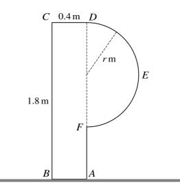
The diagram shows the cross-section ABCDEF through the centre of mass of a uniform prism which rests with AB on rough horizontal ground. ABCD is a rectangle with AB = CD = 0.4 m and BC = AD = 1.8 m. The other part of the cross-section is a semicircle with diameter DF and radius *r* m.
