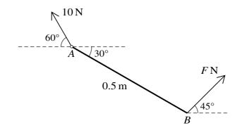
A non-uniform rod AB of length 0.5 m is freely hinged to a fixed point at A. The rod is in equilibrium at an angle of  $30^{\circ}$  with the horizontal with B below the level of A. Equilibrium is maintained by a force of magnitude F N applied at B acting at  $45^{\circ}$  above the horizontal in the vertical plane containing AB. The force exerted by the hinge on the rod has magnitude 10 N and acts at an angle of  $60^{\circ}$  above the horizontal (see diagram).
