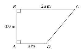
The diagram shows the cross-section *ABCD* through the centre of mass of a uniform solid prism. AB = 0.9 m, BC = 2a m, AD = a m and angle *ABC* = angle *BAD* = 90°.
