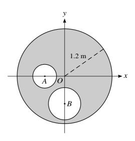
A uniform circular disc has centre *O* and radius 1.2 m. The centre of the disc is at the origin of *x*- and *y*-axes. Two circular holes with centres at *A* and *B* are made in the disc (see diagram). The point *A* is on the negative *x*-axis with OA = 0.5 m. The point *B* is on the negative *y*-axis with OB = 0.7 m. The hole with centre *A* has radius 0.3 m and the hole with centre *B* has radius 0.4 m. Find the distance of the centre of mass of the object from
