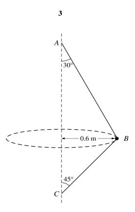
One end of a light inextensible string is attached to a fixed point *A*. The string passes through a smooth bead *B* of mass 0.3 kg and the other end of the string is attached to a fixed point *C* vertically below *A*. The bead *B* moves with constant speed in a horizontal circle of radius 0.6 m which has its centre between *A* and *C*. The string makes an angle of 30° with the vertical at *A* and an angle of 45° with the vertical at *C* (see diagram).
