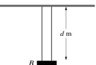
Two light elastic strings each have one end attached to a fixed horizontal beam. One string has natural length 0.6 m and modulus of elasticity 12 N; the other string has natural length 0.7 m and modulus of elasticity 21 N. The other ends of the strings are attached to a small block B of weight W N. The block hangs in equilibrium d m below the beam, with both strings vertical (see diagram).
