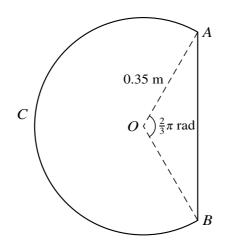
A uniform lamina ABC is in the form of a major segment of a circle with centre O and radius 0.35 m. The straight edge of the lamina is AB, and angle  $AOB = \frac{2}{3}\pi$  radians (see diagram).
