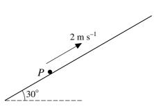
A particle *P* of mass 0.2 kg is projected with velocity  $2 \text{ m s}^{-1}$  upwards along a line of greatest slope on a plane inclined at 30° to the horizontal (see diagram). Air resistance of magnitude 0.5*v* N opposes the motion of *P*, where  $v \text{ m s}^{-1}$  is the velocity of *P* at time *t* s after projection. The coefficient of friction between *P* and the plane is  $\frac{1}{2\sqrt{3}}$ . The particle *P* reaches a position of instantaneous rest when t = T.
