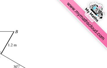
A uniform rod AB has weight 15 N and length 1.2 m. The end A of the rod is in contact with a rough plane inclined at 30° to the horizontal, and the rod is perpendicular to the plane. The rod is held in equilibrium in this position by means of a horizontal force applied at B, acting in the vertical plane containing the rod (see diagram).
