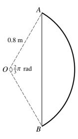
A bow consists of a uniform curved portion AB of mass 1.4 kg, and a uniform taut string of mass m kg which joins A and B. The curved portion AB is an arc of a circle centre O and radius 0.8 m. Angle AOB is  $\frac{2}{3}\pi$  radians (see diagram). The centre of mass of the bow (including the string) is 0.65 m from O. Calculate m.
