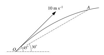
A particle P is projected from a point O with initial speed  $10 \,\mathrm{m\,s^{-1}}$  at an angle of  $45^\circ$  above the horizontal. P subsequently passes through the point A which is at an angle of elevation of  $30^\circ$  from O (see diagram). At time t s after projection the horizontal and vertically upward displacements of P from O are x m and y m respectively.
