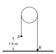
Particles A and B, of masses 0.35 kg and 0.15 kg respectively, are attached to the ends of a light inextensible string which passes over a fixed smooth pulley. The system is at rest with B held on the horizontal floor, the string taut and its straight parts vertical. A is at a height of 1.6 m above the floor (see diagram). B is released and the system begins to move; B does not reach the pulley. Find
