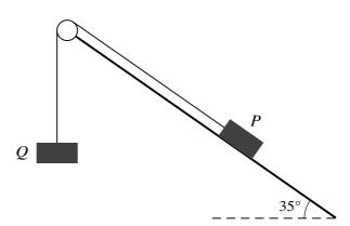
Blocks P and Q, of mass  $m \log a$  and 5 kg respectively, are attached to the ends of a light inextensible string. The string passes over a small smooth pulley which is fixed at the top of a rough plane inclined at  $35^{\circ}$  to the horizontal. Block P is at rest on the plane and block Q hangs vertically below the pulley (see diagram). The coefficient of friction between block P and the plane is 0.2. Find the set of values of P of which the two blocks remain at rest.
