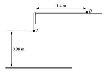
Particles A and B have masses 0.32 kg and 0.48 kg respectively. The particles are attached to the ends of a light inextensible string which passes over a small smooth pulley fixed at the edge of a smooth horizontal table. Particle B is held at rest on the table at a distance of 1.4 m from the pulley. A hangs vertically below the pulley at a height of 0.98 m above the floor (see diagram). A, B, the string and the pulley are all in the same vertical plane. B is released and A moves downwards.
