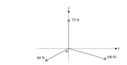
Three coplanar forces of magnitudes 68 N, 75 N and 100 N act at an origin O, as shown in the diagram. The components of the three forces in the positive *x*-direction are -60 N, 0 N and 96 N, respectively. Find
