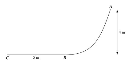
ABC is a vertical cross-section of a surface. The part of the surface containing AB is smooth and A is 4 m higher than B. The part of the surface containing BC is horizontal and the distance BC is 5 m (see diagram). A particle of mass 0.8 kg is released from rest at A and slides along ABC. Find the speed of the particle at C in each of the following cases.
