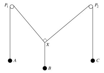
The diagram shows three particles A, B and C hanging freely in equilibrium, each being attached to the end of a string. The other ends of the three strings are tied together and are at the point X. The strings carrying A and C pass over smooth fixed horizontal pegs  $P_1$  and  $P_2$  respectively. The weights of A, B and C are 5.5 N, 7.3 N and W N respectively, and the angle  $P_1XP_2$  is a right angle. Find the angle  $AP_1X$  and the value of W.
