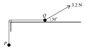
Particles P and Q, of masses 0.2 kg and 0.5 kg respectively, are connected by a light inextensible string. The string passes over a smooth pulley at the edge of a rough horizontal table. P hangs freely and Q is in contact with the table. A force of magnitude 3.2 N acts on Q, upwards and away from the pulley, at an angle of  $30^{\circ}$  to the horizontal (see diagram).
