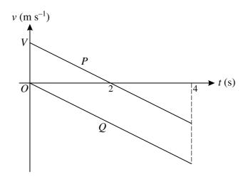
Two particles P and Q move vertically under gravity. The graphs show the upward velocity  $v \, \text{m s}^{-1}$  of the particles at time  $t \, \text{s}$ , for  $0 \leq t \leq 4$ . P starts with velocity  $V \, \text{m s}^{-1}$  and Q starts from rest.
