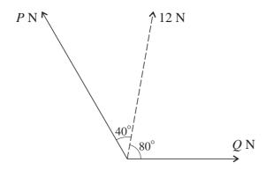
Two forces have magnitudes PN and QN. The resultant of the two forces has magnitude 12N and acts in a direction  $40^{\circ}$  clockwise from the force of magnitude PN and  $80^{\circ}$  anticlockwise from the force of magnitude QN (see diagram). Find the value of Q. [4]
