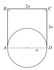
Three identical uniform rods, AB, BC and CD, each of mass M and length 2a, are rigidly joined to form three sides of a square. A uniform circular disc, of mass  $\frac{2}{3}M$  and radius a, has the opposite ends of one of its diameters attached to A and D respectively. The disc and the rods all lie in the same plane (see diagram). Find the moment of inertia of the system about the axis AD. [6]
