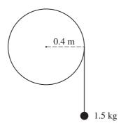
A uniform disc of radius 0.4 m is free to rotate without friction in a vertical plane about a horizontal axis through its centre. The moment of inertia of the disc about the axis is  $0.2 \,\mathrm{kg}\,\mathrm{m}^2$ . One end of a light inextensible string is attached to a point on the rim of the disc and the string is wound round the rim. The other end of the string is attached to a particle of mass 1.5 kg which hangs freely (see diagram). The system is released from rest. Find
